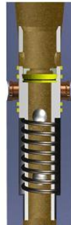
Tool can be hydraulically reset (unlocked) downhole by dropping 2 steel deactivation balls. Locking Ball and Activation Ball will Shear and FLOW to BIT resumed.
