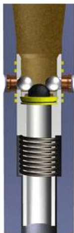
Tool can be hydraulically reset (unlocked) downhole by dropping 2 steel deactivation balls. Locking Ball and Activation Ball will Shear and FLOW to BIT resumed.
