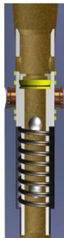
Balls Sheared Thru Seat Tool Reset
