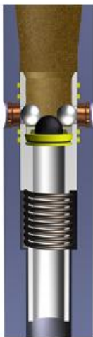
De-Activation Balls Dropped PRESSURE UP
