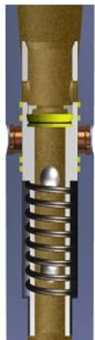
Balls Sheared Thru Seat Tool Reset
